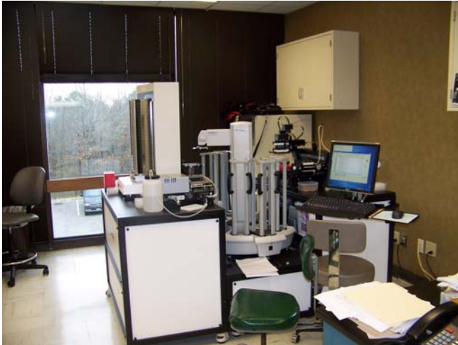
Figure 6. Right Side View of System. The Twister II robotic arm/gripper and storage stacks are seen, along with the LPX44 plate hotel and computer console.
