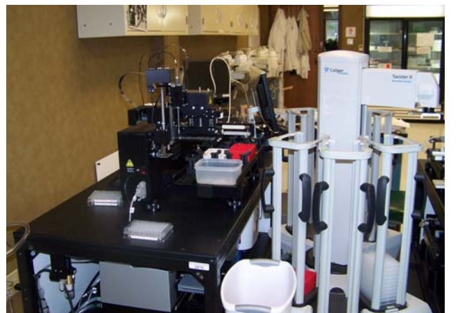
Figure 5. Left Side View of System. The Twister II robotic arm/gripper and storage racks are seen in the center section, while the Precision XS is seen on the top level of one of the end-unit tables.
